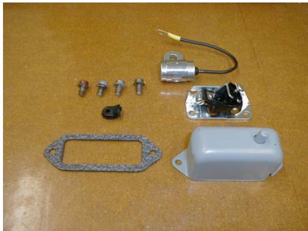
Points and condenser ready for installation
