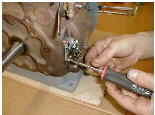
Installing Points Assembly
